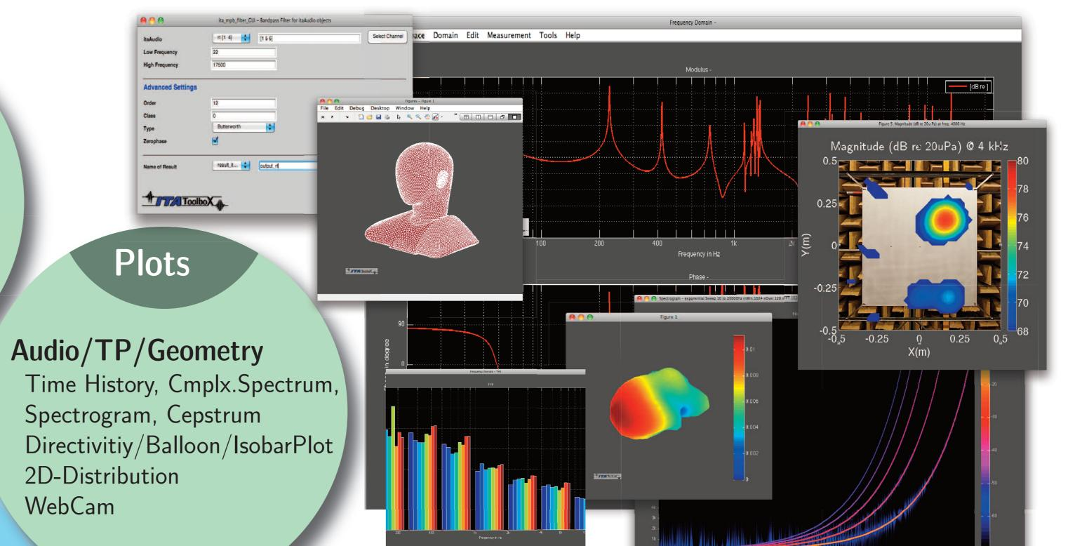
Excitation Signals:Sweep/MLS Impedances:Loudspeaker,Plate Two-Port:Mass-Spring-Damper Room Impulse Responses Geometry/Mesh
